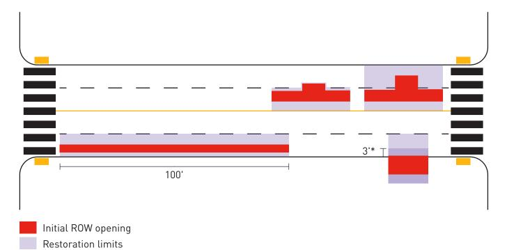
\*3' max pavement restoration on non-arterial street or arterial street with on-street parking. On arterial streets without on-street parking, restore to lane line.
