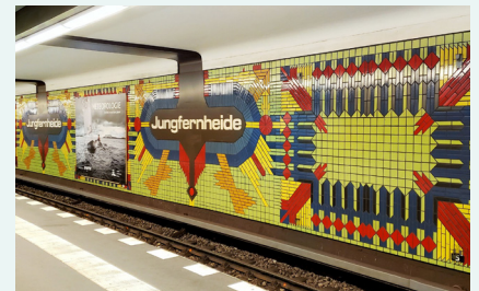
Artwork that runs the length of the platform helps user on board to recognize what platform they have arrived at without the need for signs.
