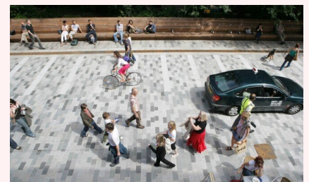
A shared street design provides ample space for pedestrians, bicyclists, and seating, while accommodating slow moving vehicles for local access.
