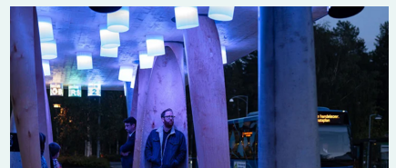
Color-changing feature lighting communicates which bus route is arriving without having to read a sign.
