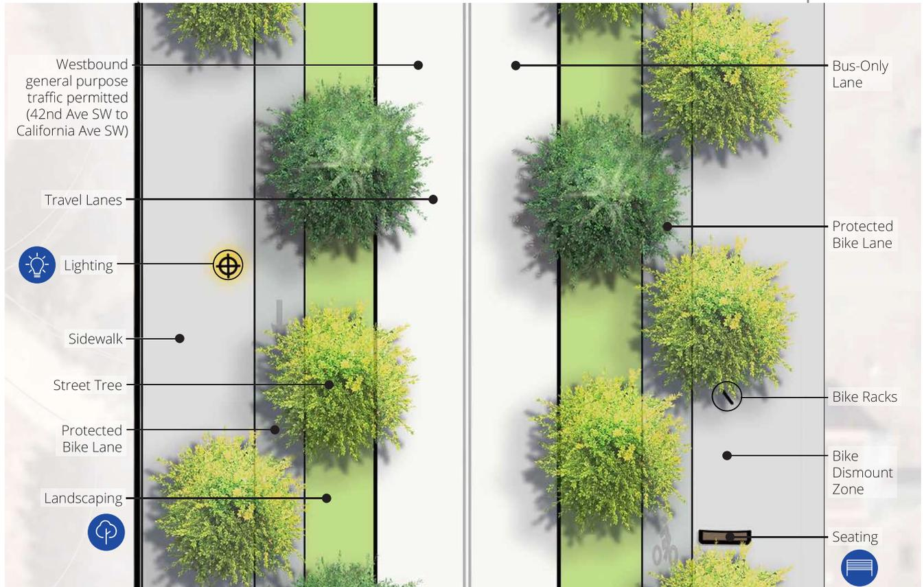
Proposed SW Alaska St section (1) looking east with plan enlargement
