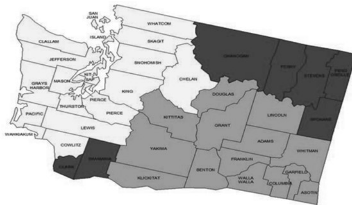
ZONE 1 HIGH POTENTIAL (GREATER THAN 4 pCi/L) [Red/Darkest] ZONE 2 MODERATE POTENTIAL (FROM 2 TO 4 pCi/L) [Orange/Midrange] ZONE 3 LOW POTENTIAL (LESS THAN 2 pCi/L) [Yellow/Lightest]
