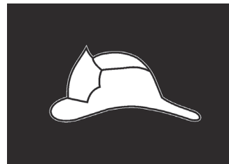
FIGURE 403.6.1.6.5 FIRE SERVICE ACCESS ELEVATOR SYMBOL
