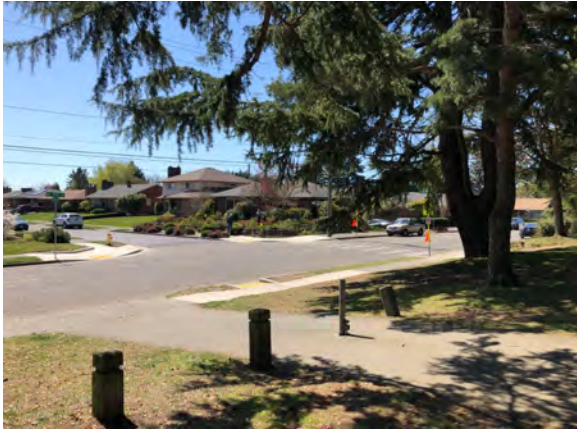
Improve accessible entrance from NE 70 th St. Match grade to sidewalk. Regrade and replace asphalt with concrete walk to restrooms.
