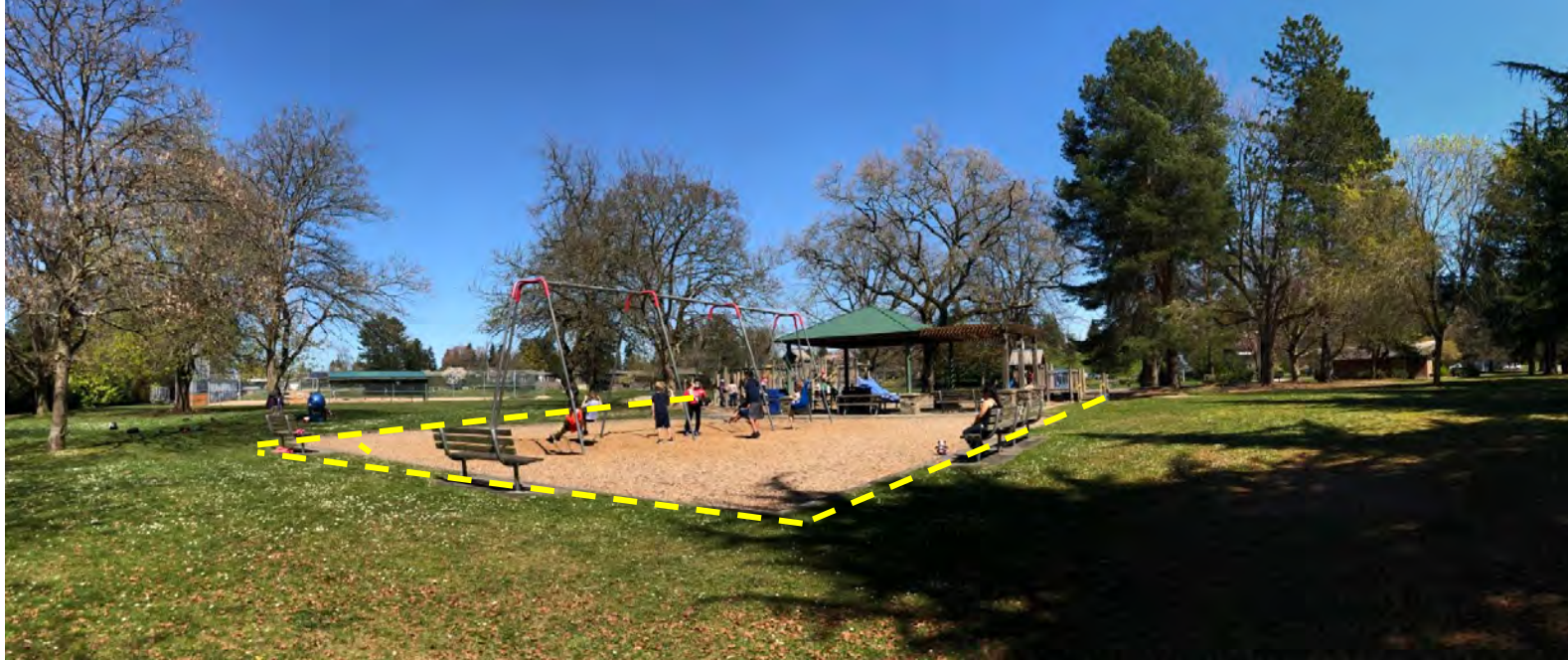
Existing tall swing takes up the whole play pod. Toddler bucket swing exceed maximum 8' high. Lack of accessible route to existing benches.
