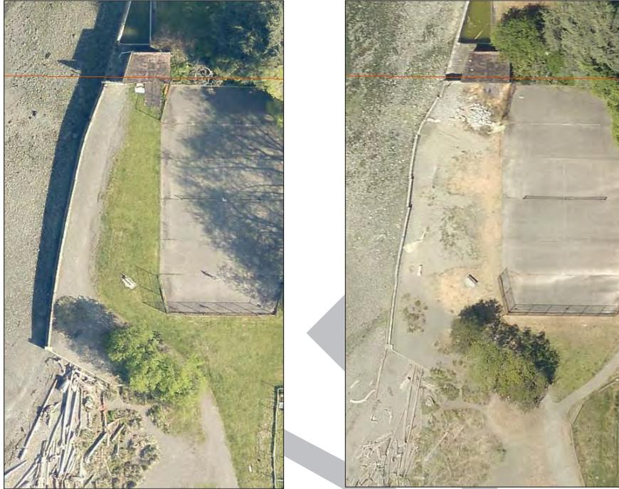
Satellite images of the Lowman Beach Park seawall in 2015, left, and 2017, right, showing the failure of the northern segment of the seawall over time. Source: King County iMap.
