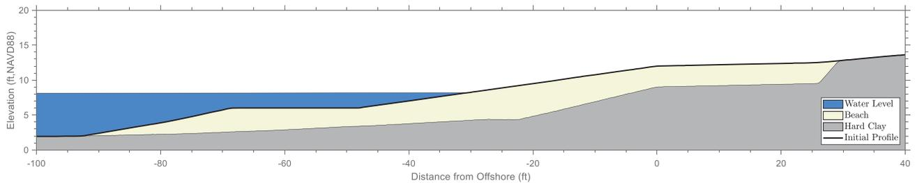
Figure 1. Typical Beach Design Profile, After Construction
