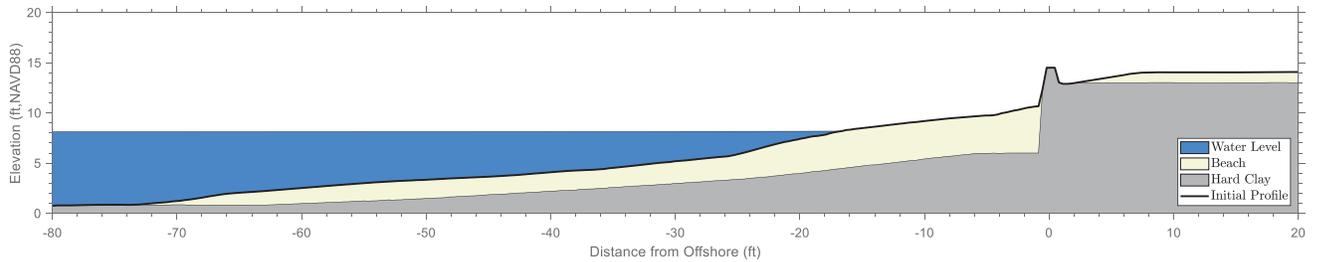
**Figure 2. Beach design profile in front of the new Seawall, After Construction**
