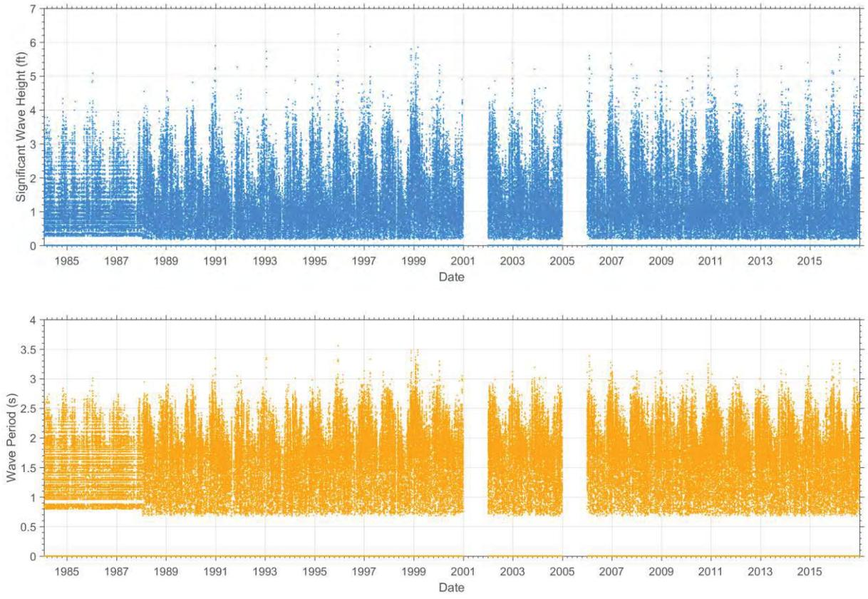
**Figure 3. Simulated Significant Wave Height and Wave Period Time Series offshore of the park.**
