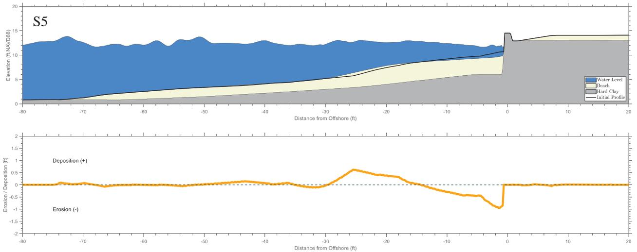
**Figure 14. Seawall-Beach Profile Response Under Storm Wave Conditions and 100-Year SWL Event**
