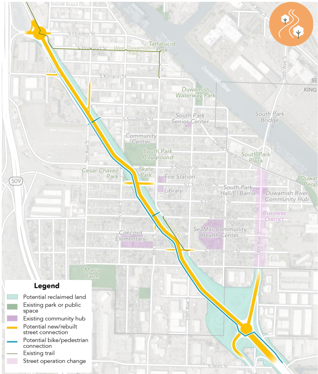
Figure 10: Concept Layout for Narrower Boulevard between S Holden St and 14 th Ave S
