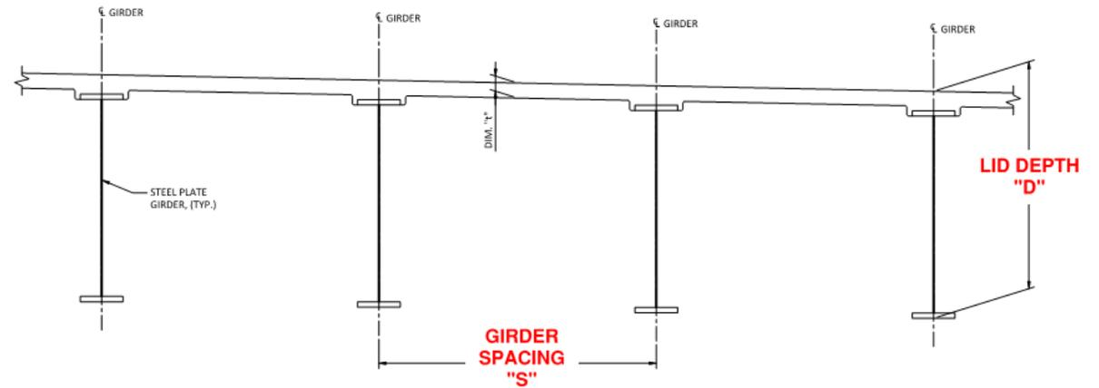
Typical Section – Steel Plate Girder
