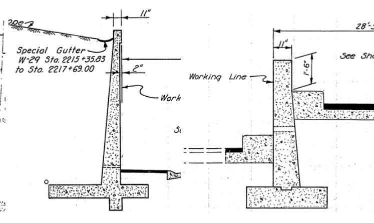
Cantilever Retaining Walls
