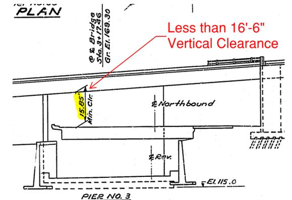
WSDOT Design Manual M22-01.16 720.03(5)(b)(1): **16.5-ft minimum clearance** for new bridge structures.
