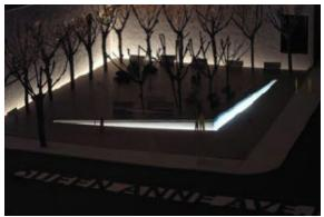
Overall, the design presents a convex light corner at the edge of the park counterbalanced with a concave light corner defined by the two existing walls. Light shines upward, along the length of existing walls, illuminating the sides of the park. New walls on the sidewalk edge of the park are lit to create a glowing Light Corner. Lights can be programmed to change color for special events, holidays, and changing seasons.
