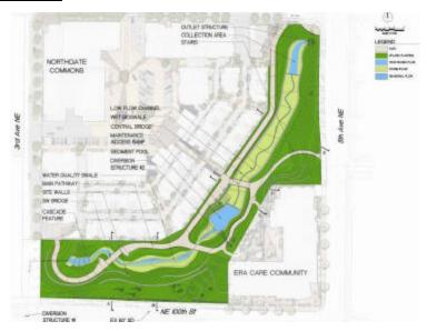
The proposed plan uses both channels and swales to remove pollutants on two different scales in a three step process.
