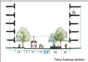
is a curb along at the northwest along Terry Ave, but the intersection of Harrison and Terry is curbless; bollards are used to separate the pedestrian zone. The east side of the street would be curbless with a swale for water collection.
