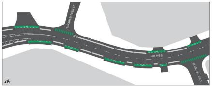
• One-way protected bike lanes on both sides of the street, with transitions at new all way stop at Nevada St.
