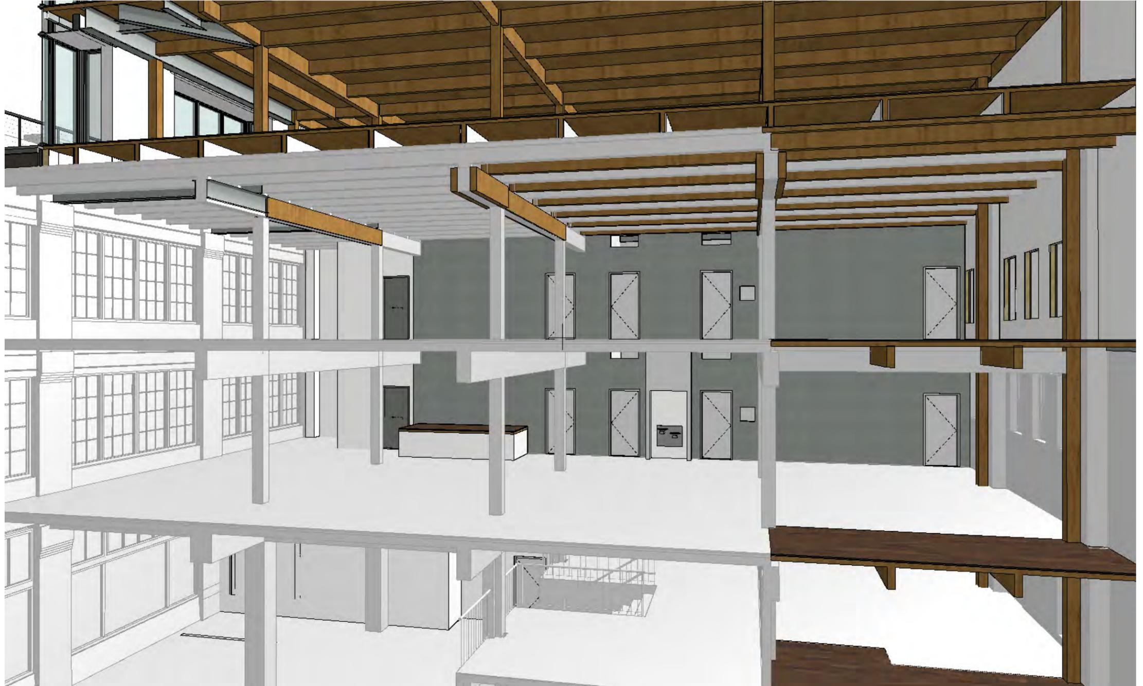
Section perspective looking east showing new structural elements
