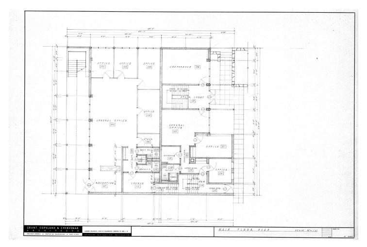
FIGURE 80: FIRST FLOOR PLAN (GRANT, COPELAND AND CHERVENAK, 1959)
