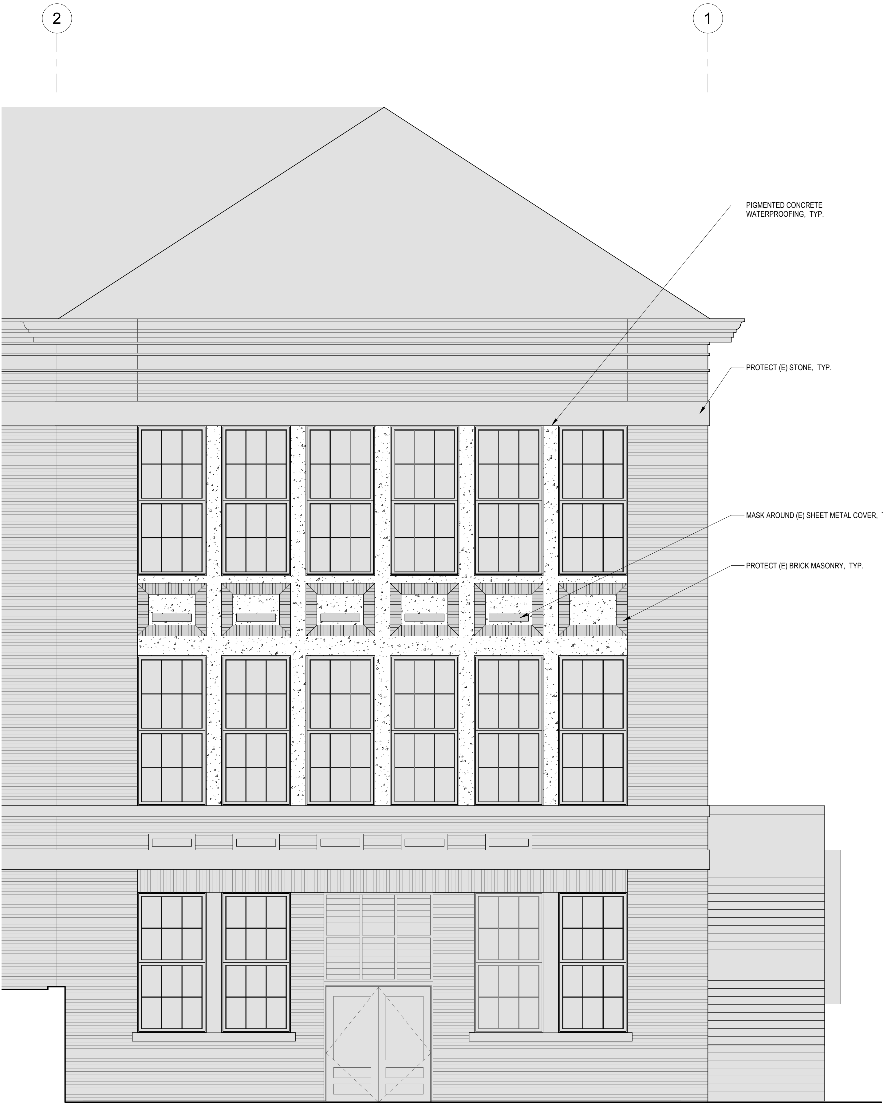
2 Enlarged West Elevation - Concrete Repairs Southwest 1/4" = 1'-0"
