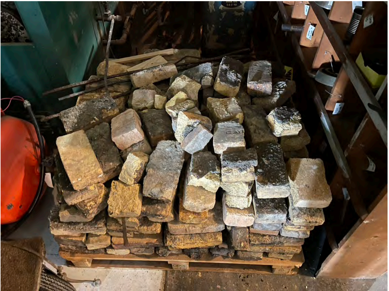
Bricks and Rebar Removed from Boiler Floor/Ash Hopper Above
