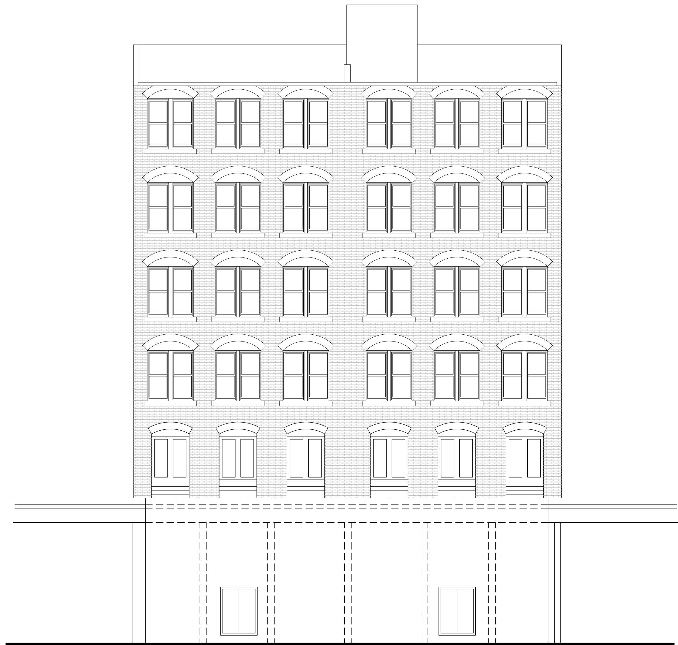
PROPOSED EAST EXTERIOR ELEVATION 2 1/8" = 1'-0" A3.2
