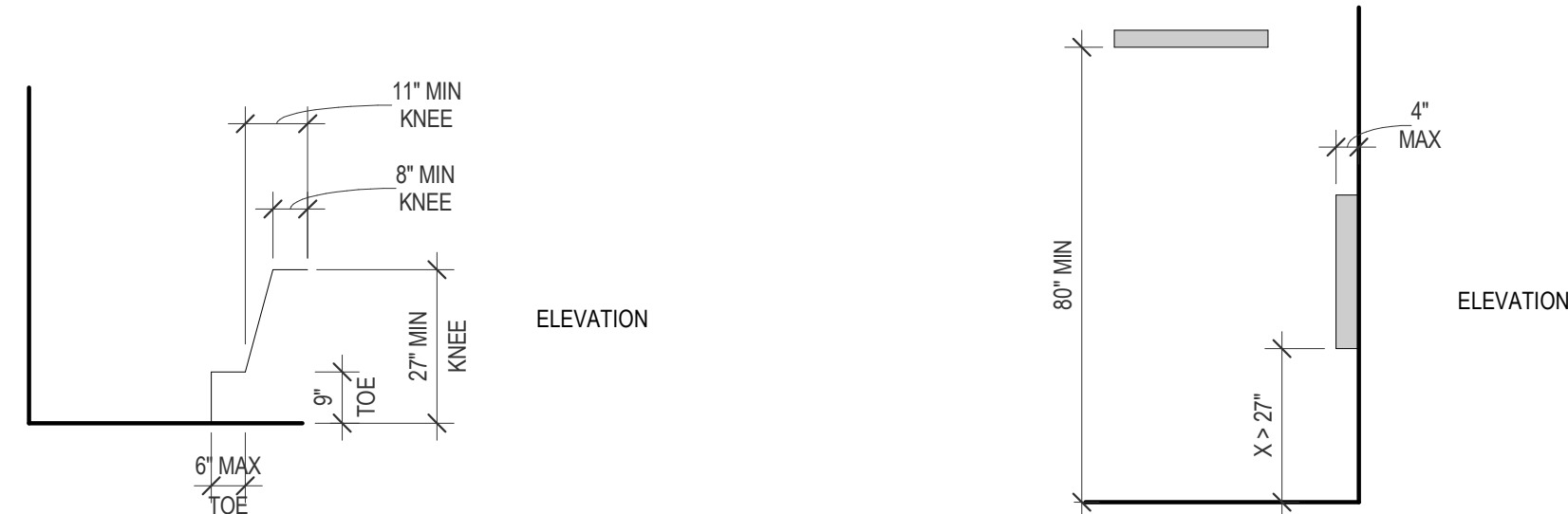
KNEE AND TOE CLEARANCE PER ICC A117.1 SECTION 306 SCALE: 3/8" = 1'-0"
