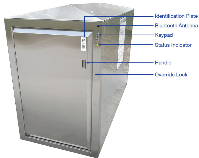
Figure 9.0: G7 Bike Locker model and its features
