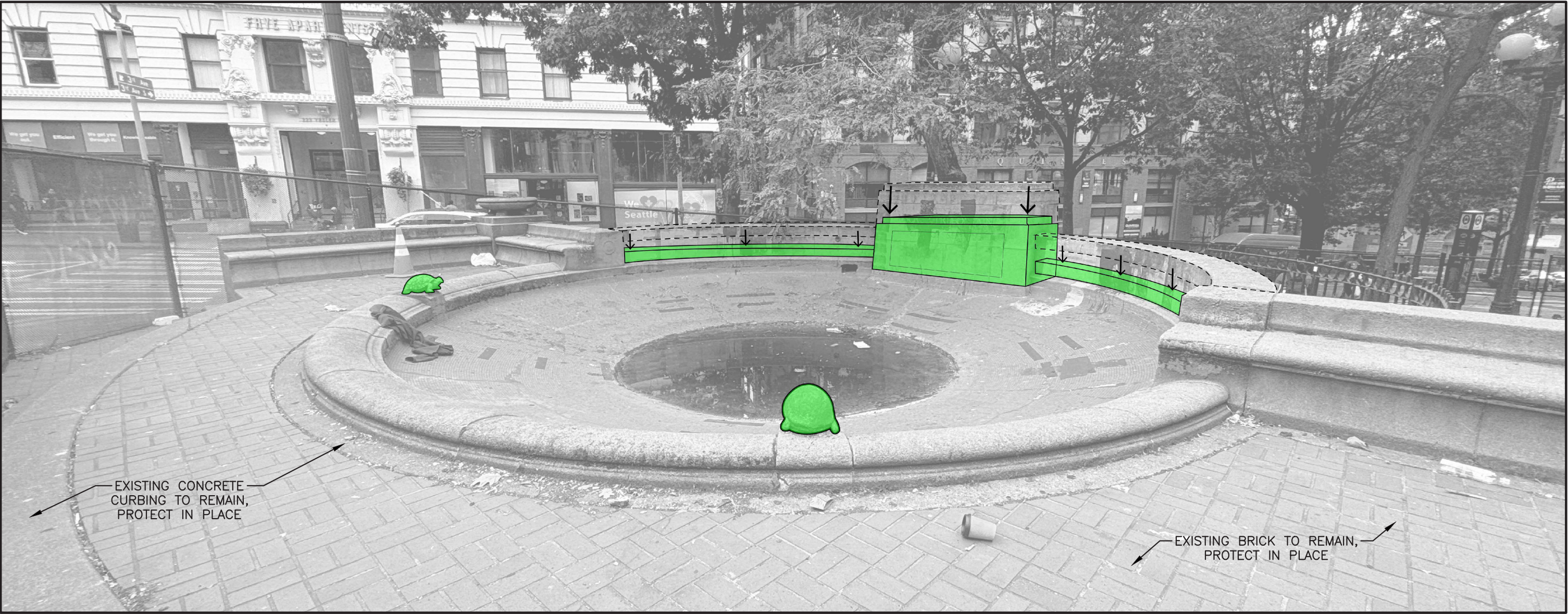
03 EXISTING FOUNTAIN SELECTIVE STONE RESTORATION DIAGRAM SCALE: NTS
