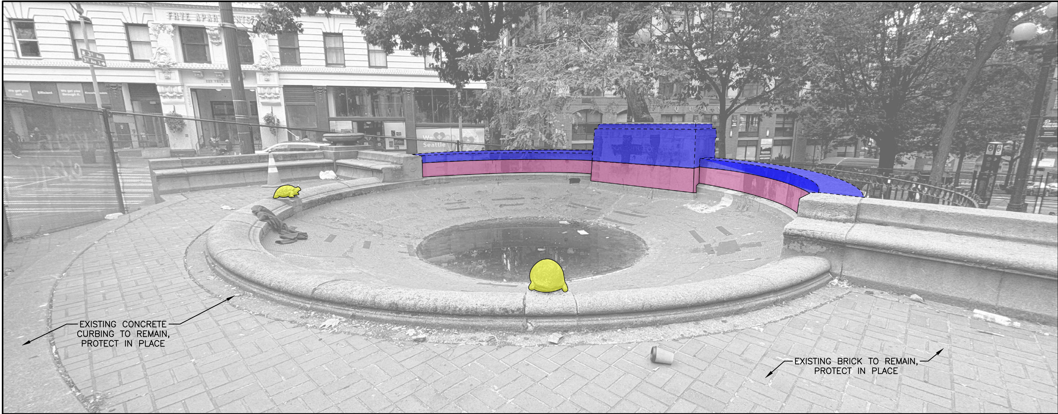
01 EXISTING FOUNTAIN SELECTIVE DEMOLITION DIAGRAM SCALE: NTS
