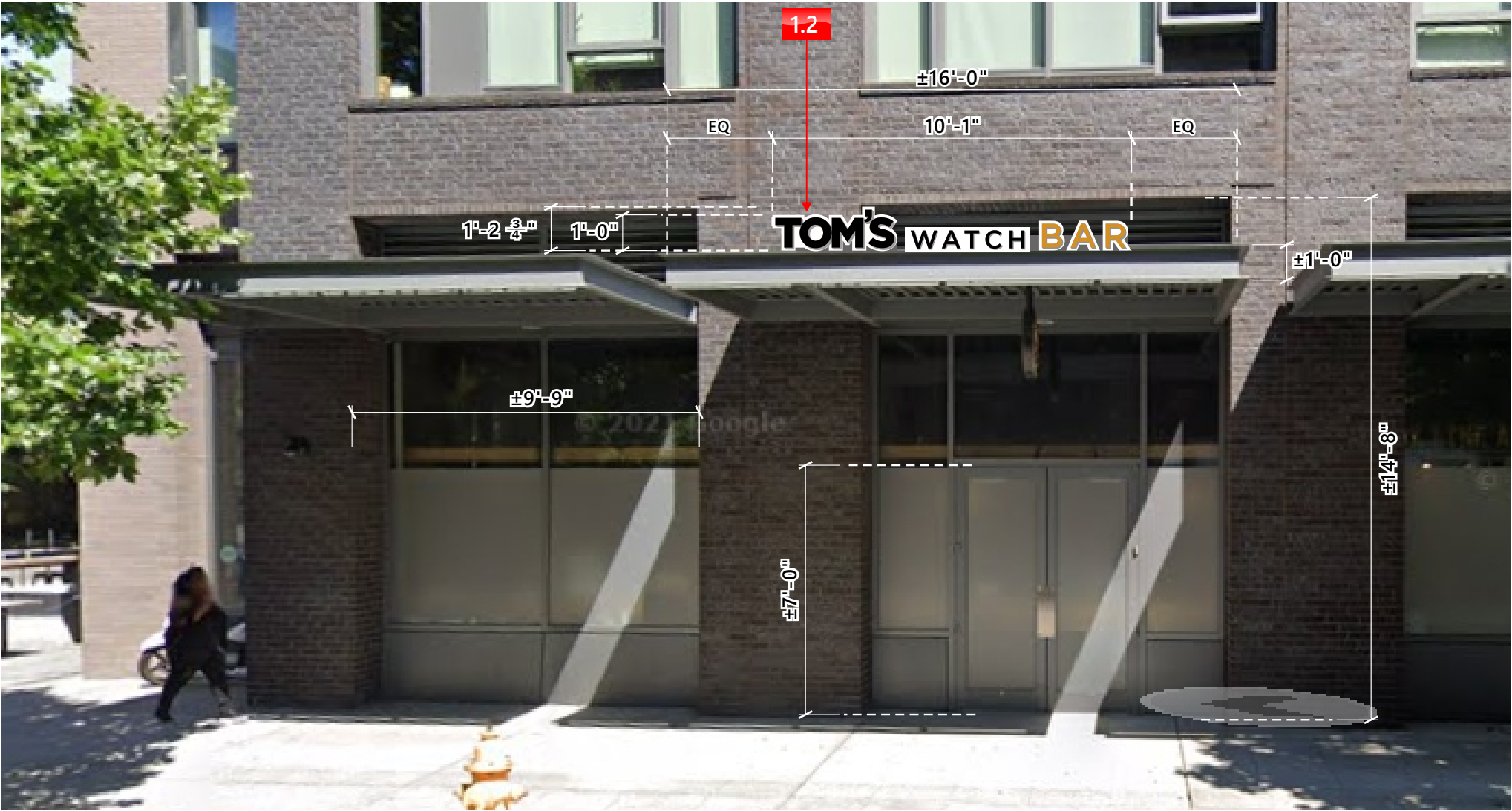
PROPOSED HALO ILLUMINATED CHANNEL LETTERS w/ BACKER PANEL ON RACEWAY
