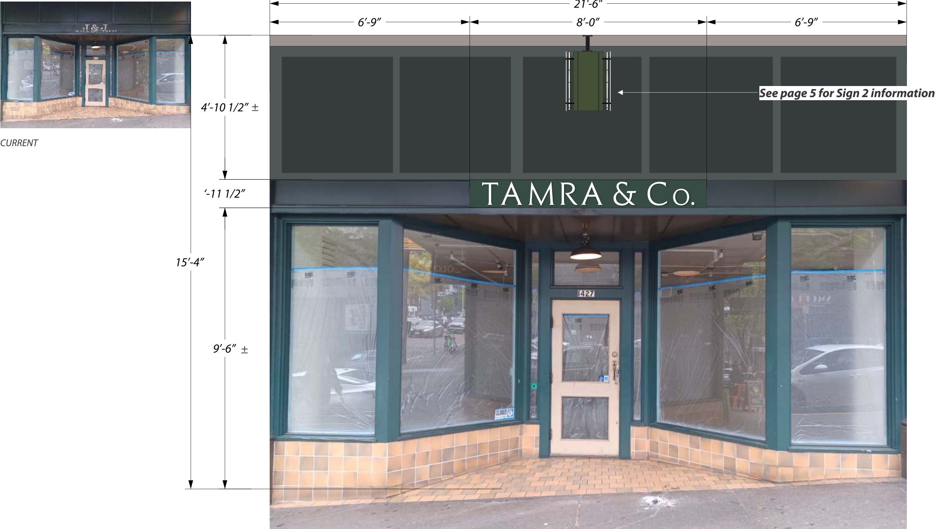
Sign 1: Non-Illuminated FCO Letterset Panel Scope: Removal and disposal of existing panel, manufacture and install new panel
