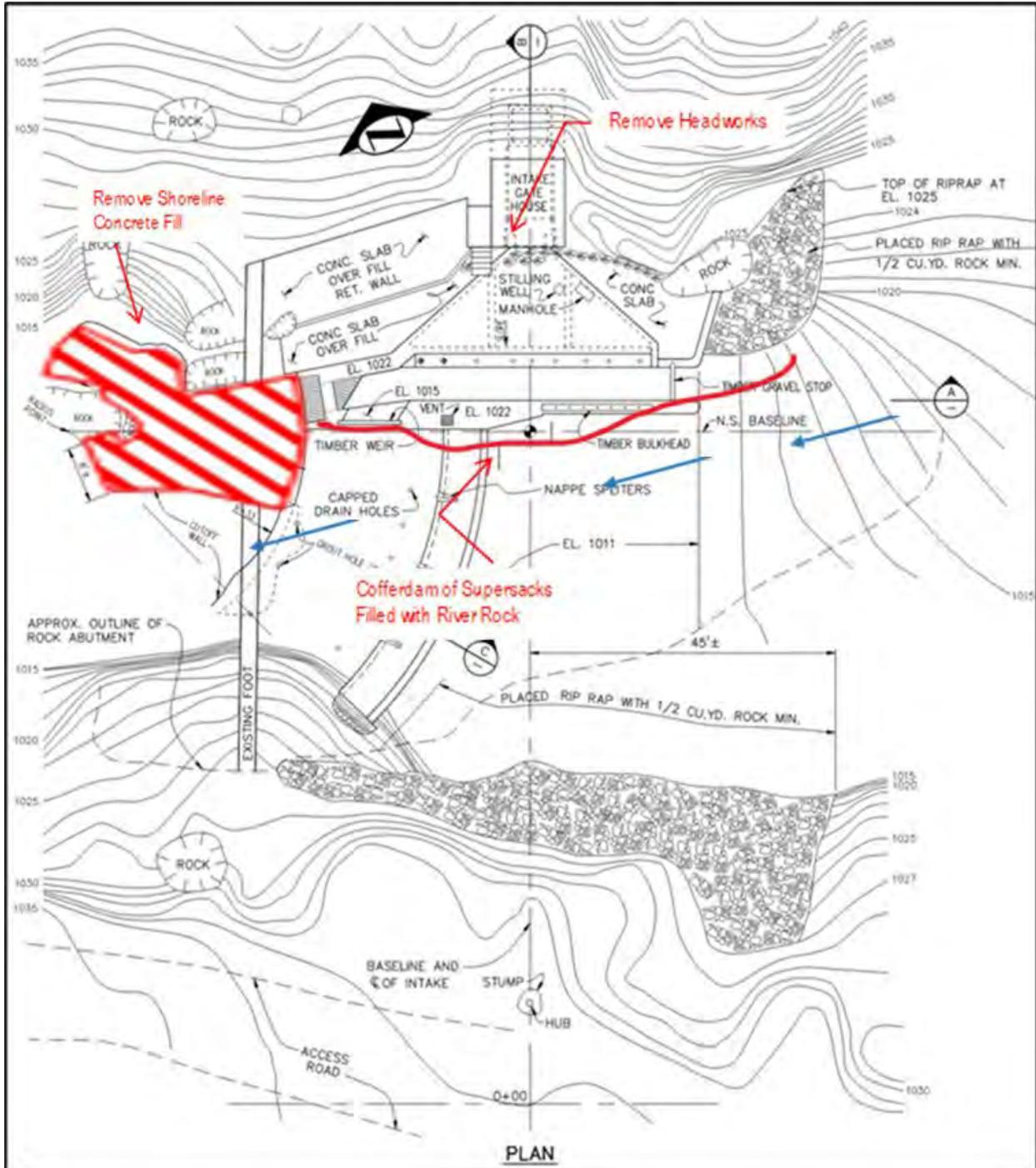
Figure 2.2-6. Shoreline Concrete Fill Removal - Site Plan.
