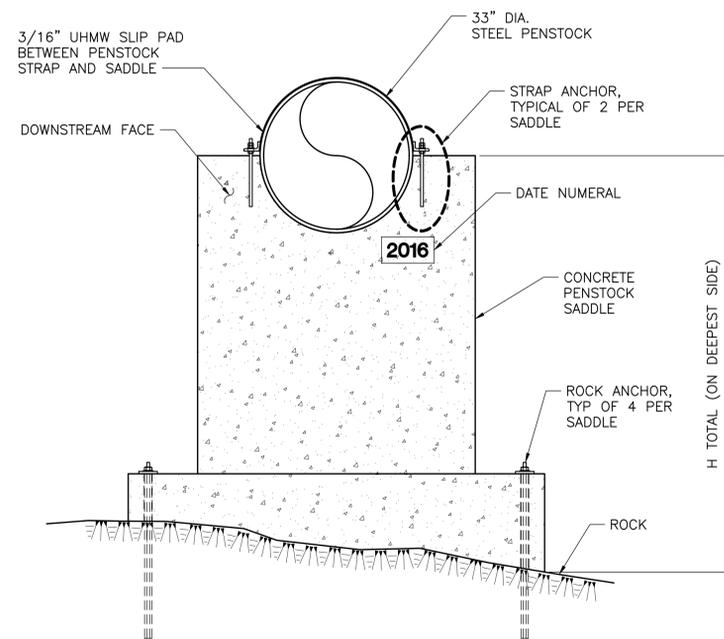
NOTE: SEE DETAILS 1/C-10 AND 2/C-10 FOR SADDLE TYPE 2A, DETAILS 3/C-10 AND 4/C-10 FOR SADDLE TYPE 2B, AND DETAILS 1/C-11 AND 2/C-11 FOR SADDLE TYPE 2C.
