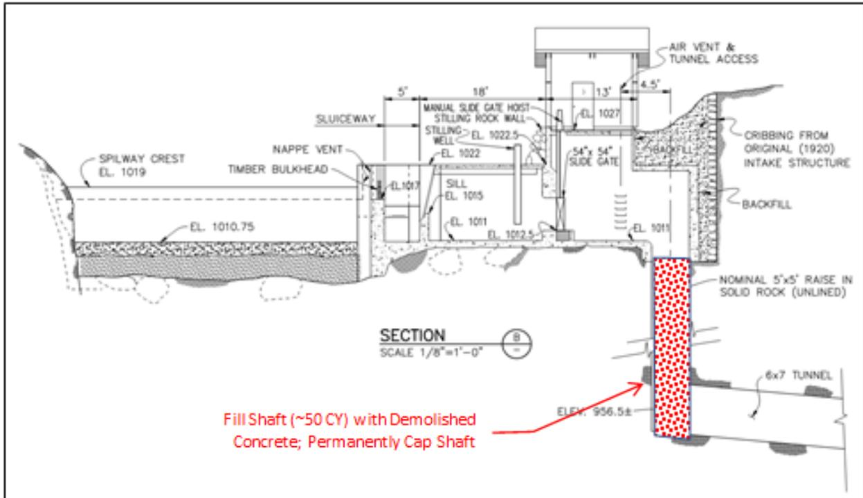
**Figure 3. Drawing of Power Tunnel Shaft with Fill**
