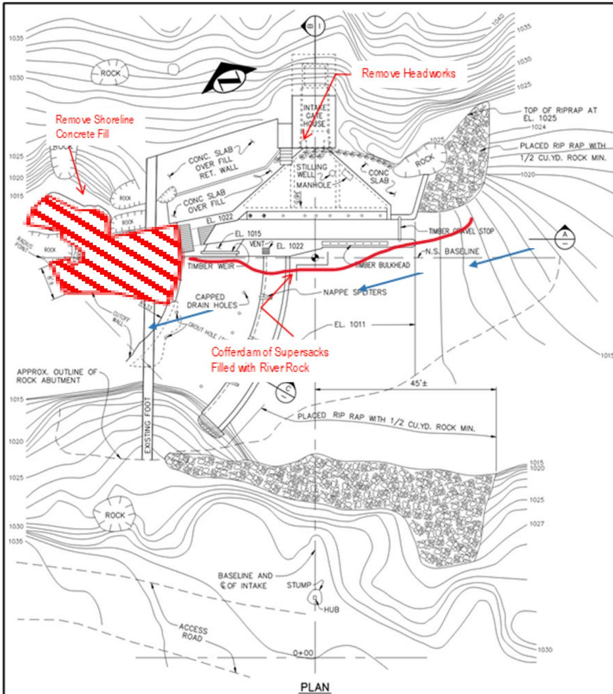
**Figure 2. Drawing of Headworks Removal**
