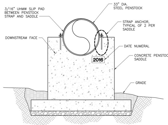
NOTE: SEE DETAILS 1/C-9 AND 2/C-9 FOR SADDLE TYPE 1A, AND DETAILS 3/C-9 AND 4/C-9 FOR TYPE 1B.
