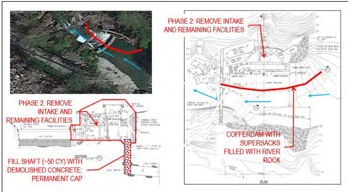
Figure 2.2-8. Conceptual site plan showing facilities to be removed during Phase 2.
