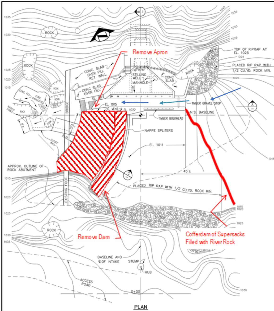
Figure 1. Drawing of Dam and Apron Removal
