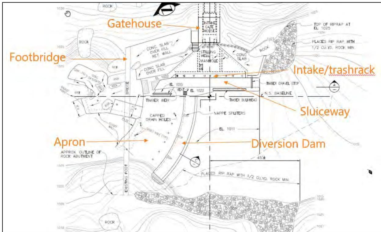
**Figure 1.1-2. Newhalem Creek Diversion Structure – existing features.**
