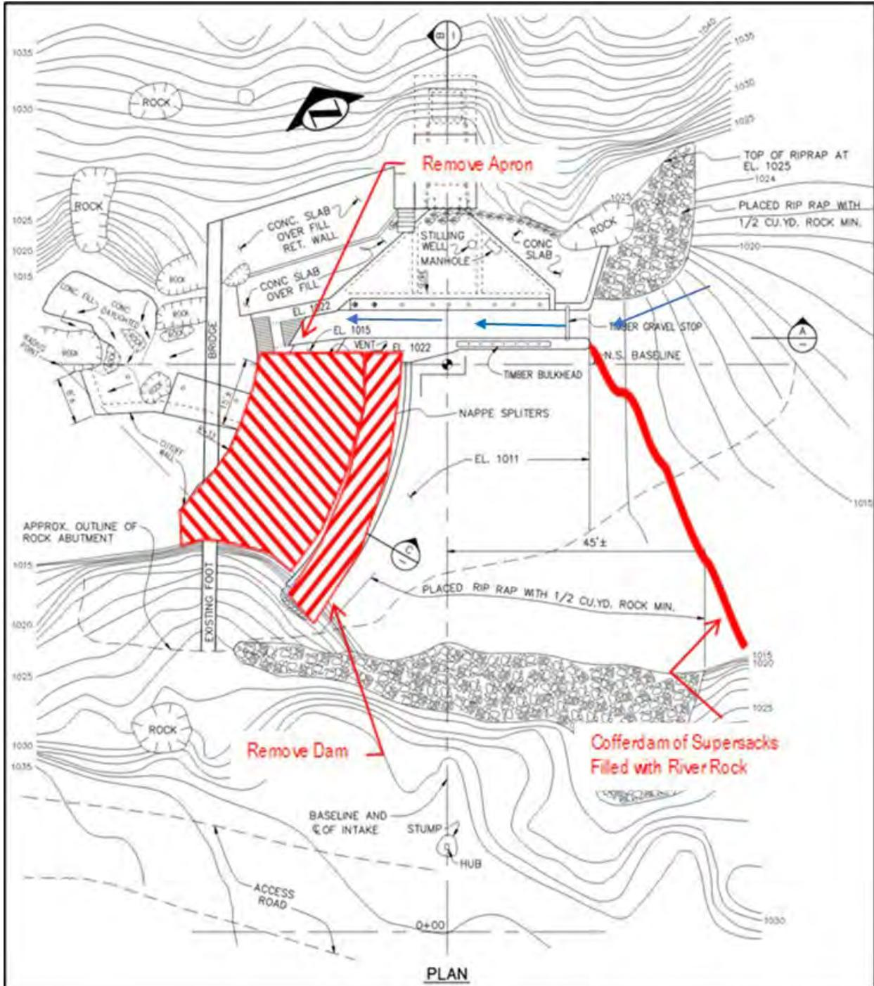
Figure 2.2-5. Dam and Apron Removal Site Plan.
