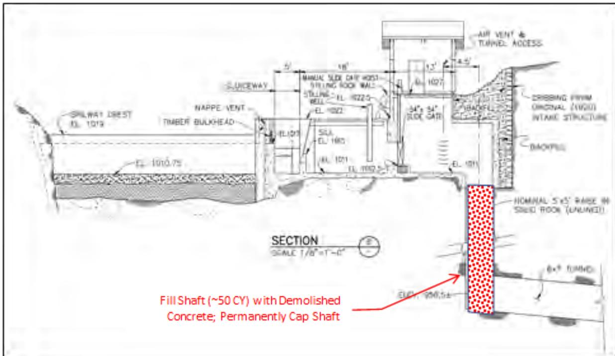
**Figure E-2. Drawing of Power Tunnel Shaft with Fill**
