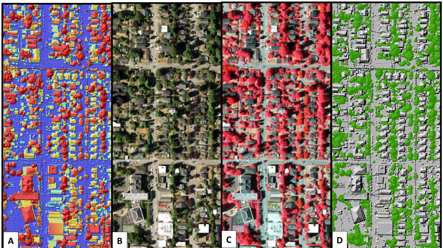
Figure 3. Example of the input data used to extract tree canopy data. LiDAR is on the left, true color imagery, CIR Imagery, and then tree canopy data on the right.
