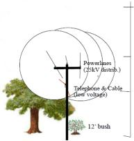
New "trim-to" distance proposed of 20'. This is being proposed by the power company at the same time the FERC has reduced their minimum clearance requirements from 2.5' to 1.5' for 125 kV lines
