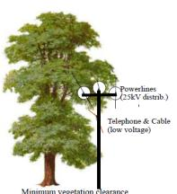
Minimum vegetation clearance which would trigger the need to start the trimming cycle (trim from distance)
