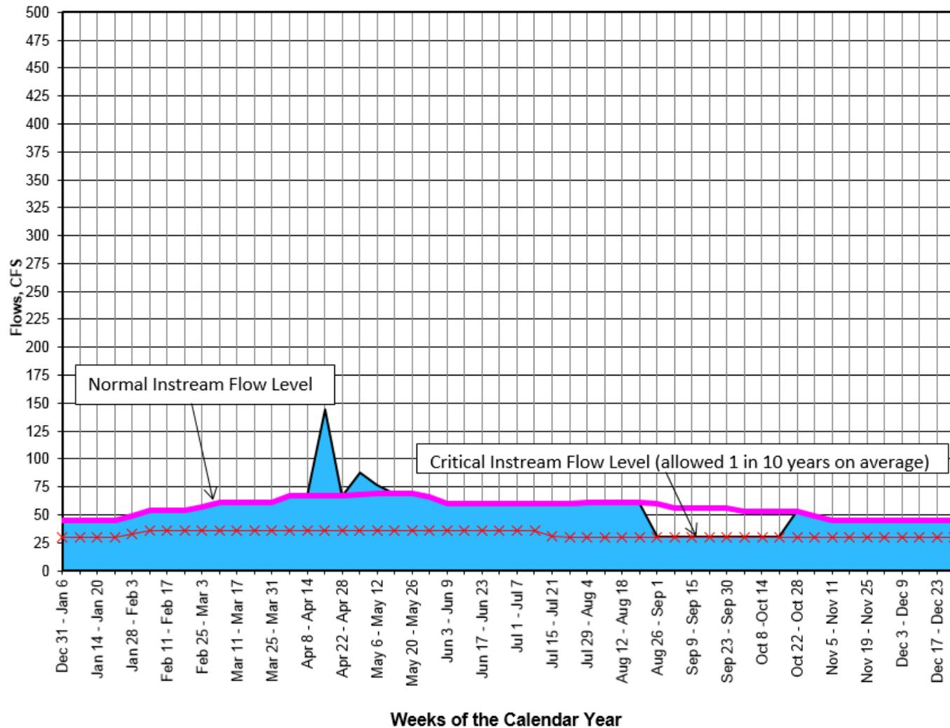
Modeled SF Tolt River minimum instream flow requirements and model output using 1987 hydrologic conditions and assuming 172 mgd system-wide demand.
