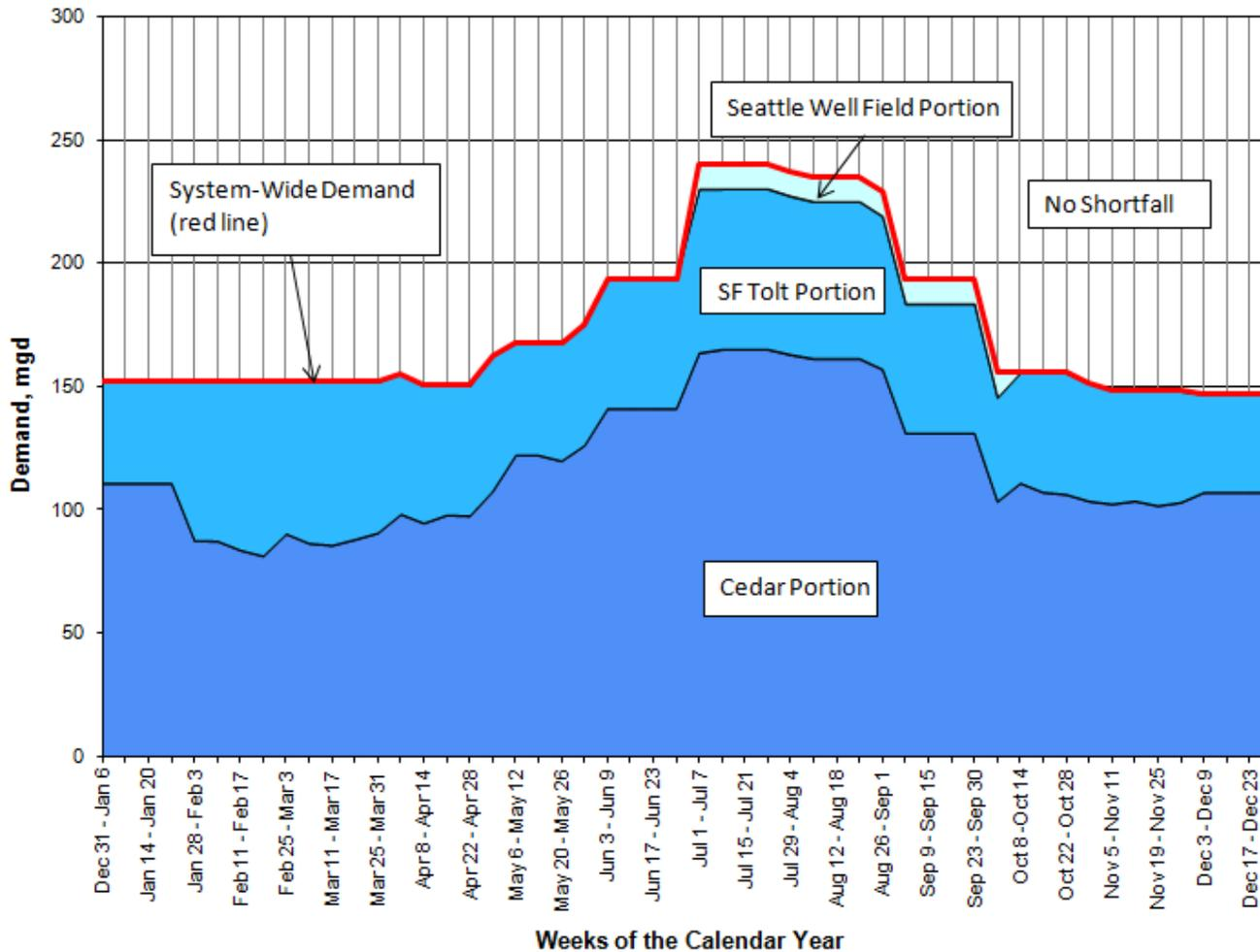
Modeled system-wide demand pattern and model output showing components of water supply sources using 1941 hydrologic conditions and assuming 172 mgd system-wide demand. No shortfall occurs in the model.
