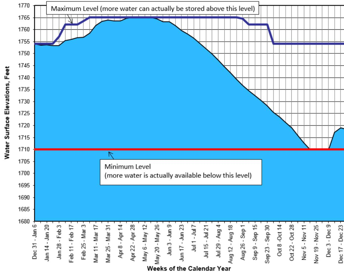
Modeled SF Tolt Reservoir operating zones and model output using 1987 hydrologic conditions and assuming 172 mgd system-wide demand. More water is available below the modeled minimum level and further investigative studies are planned to ensure reliability from water quality and treatment perspectives before changing this model assumption.
