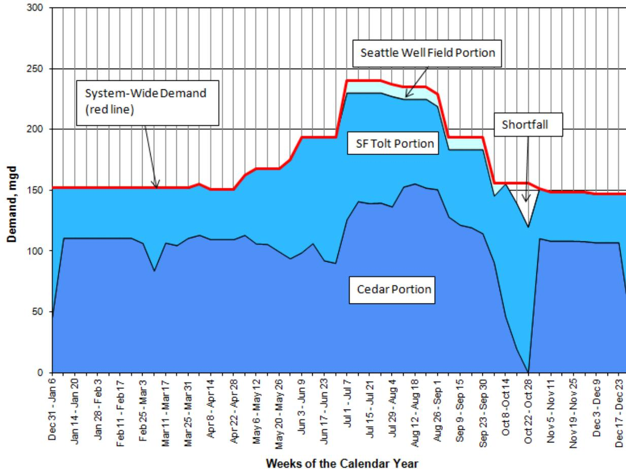
Modeled system-wide demand pattern and model output showing components of water supply sources using 2015 hydrologic conditions and assuming 172 mgd system-wide demand. Shortfall occurs in the model. Real-world we have curtailment contingency plans and emergency backup supplies.
