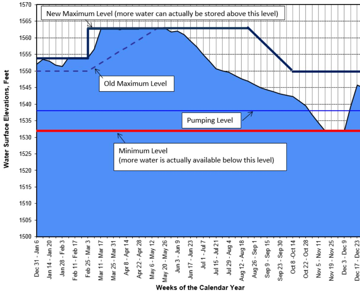
Modeled Cedar Reservoir operating zones and model output using 1987 hydrologic conditions and assuming 172 mgd system-wide demand. Modeled reservoir refill rule curve changed to capture and store more water in early spring. More water is available below the modeled minimum level and in real-world is accessible as an emergency backup source of supply.
