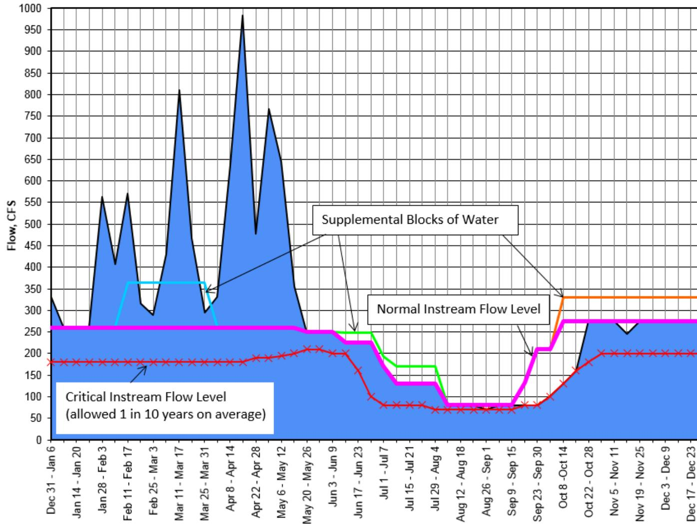
Modeled Cedar River minimum instream flow requirements and model output using 1987 hydrologic conditions and assuming 172 mgd system-wide demand.
