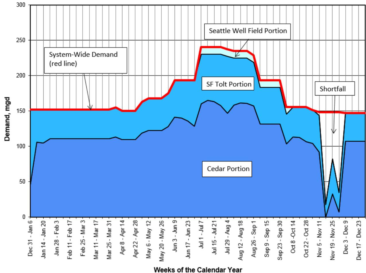
Modeled system-wide demand pattern and model output showing components of water supply sources using 1987 hydrologic conditions and assuming 172 mgd system-wide demand. Shortfall occurs in the model. Real-world we initiate curtailment contingency plans and have emergency backup water supplies.
