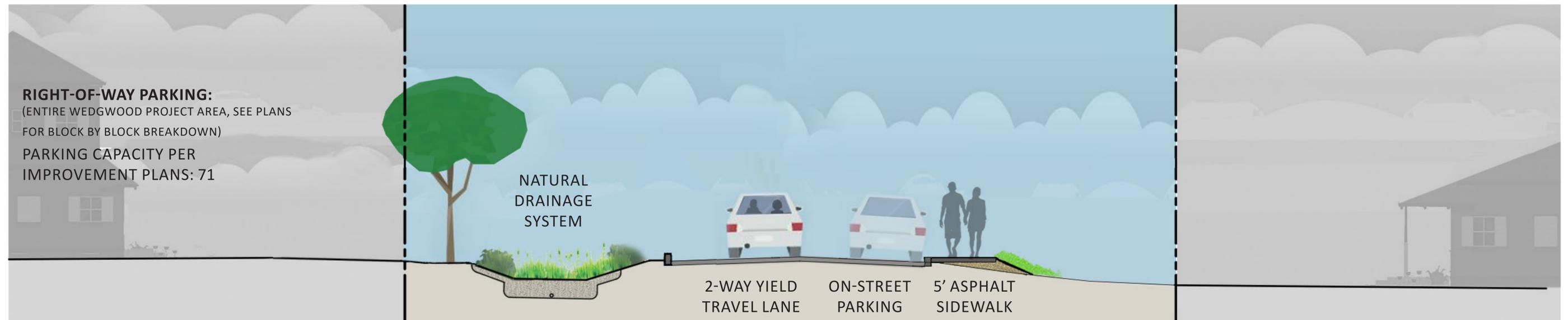
PROPOSED TYPICAL STREET SECTION WITH ASPHALT-THICKENED EDGE (CURBING AT NDS) AND NATURAL DRAINAGE SYSTEM ON SOUTH SIDE, CURB AND SIDEWALK ON NORTH SIDE
