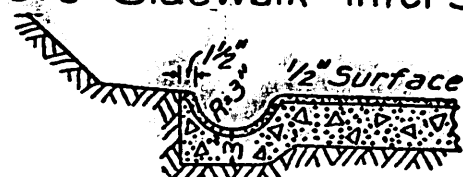
Section of Gutter with Concrete Walk CONCRETE WALKS
