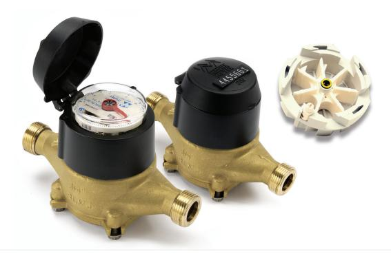
Master Meter's Multi-Jet meter exceeds the AWWA C708 standard. With sensitivity to measure water flowing as low as 1/8 gallon per minute and accuracy unaffected by common particulates and build-up that would freeze other types, you can count on our Multi-Jet technology.
