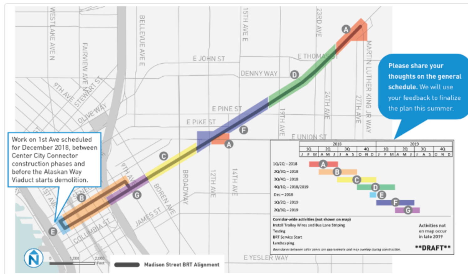
Preliminary construction phasing plan
