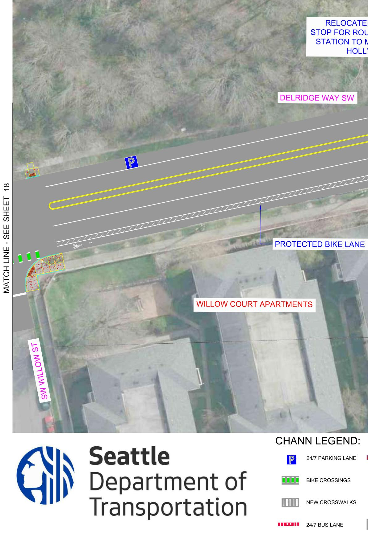
RELOCATED EX. NORTHBOUND BUS-STOP FOR ROUTE 120 WITH RAPIDRIDE STATION TO MID-BLOCK BETWEEN SW HOLLY ST AND SW WILLOW ST
