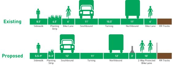
Figure 6: Typical Existing and Proposed Roadway Cross Sections
