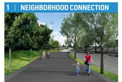
Begin walking onto the bridge via the multiuse path at the north end of North Seattle College. The bridge rises gently at a grade of approximately 4% and allows for direct connection and open sightlines.
