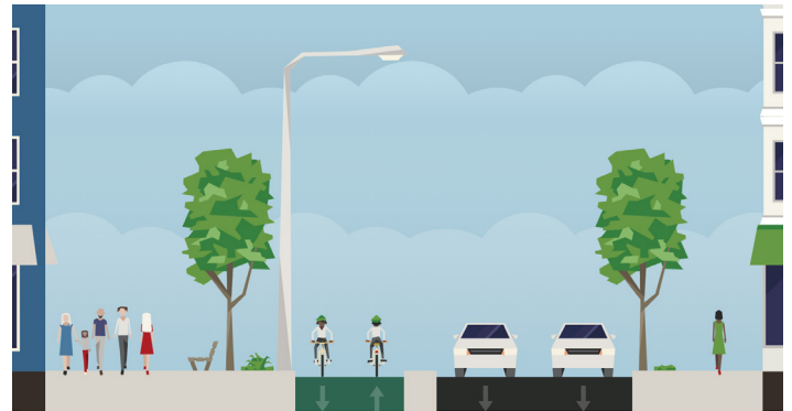
A sample street section of the new protected bike lane. In some places, the right lane will be parking; in other locations, it will function as a right-turn-only lane.
