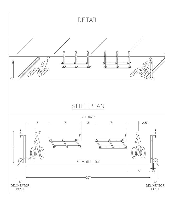
Double Bike Corral Elevation and Site Plan (Image: SDOT)
