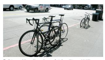
Rail type sidewalk racks on 1st Ave (Photo: SDOT)
