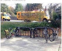
Rack does not allow use of a **u-lock** (Photo: Alta Planning + Design)
