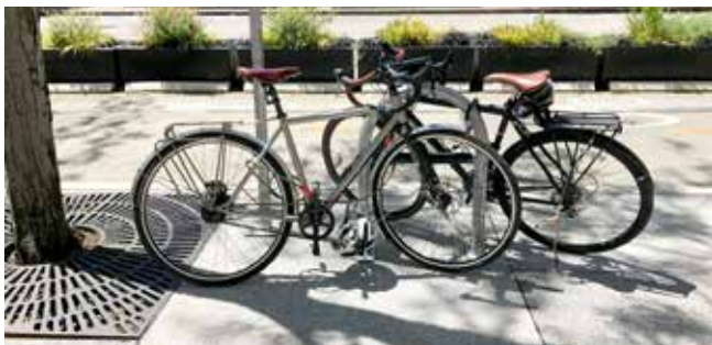
Inverted U sidewalk rack on 2nd Ave (Photo: MIG|SvR)
