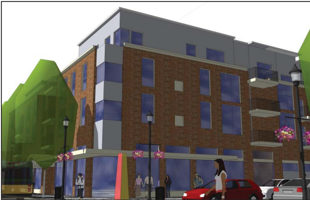
Example of a fourth floor upper level setback to reduce the apparent scale of new development
