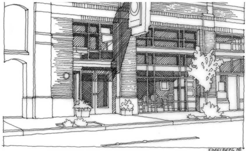
A street-facing commercial facade containing elements of traditional storefront design, including large, transparent display windows, metal framing for storefronts, and a combination of brick and masonry with channel reveals. This type of treatment is encouraged for commercial facades in new development proposals.
