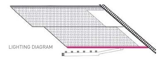
Proposed edge lighting will be utilized at the South edge of Pier 62 and the North edge of Pier 63 (in the future). This approach reinforces wayfinding paths while revealing the length and depth of the Pier structure. In addition, the edge lighting approach enhances nighttime safety and security on these structures. The Western edge of the Pier is purposefully left non-illuminated allowing occupants to take in the unobstructed nighttime view of the Sound.
