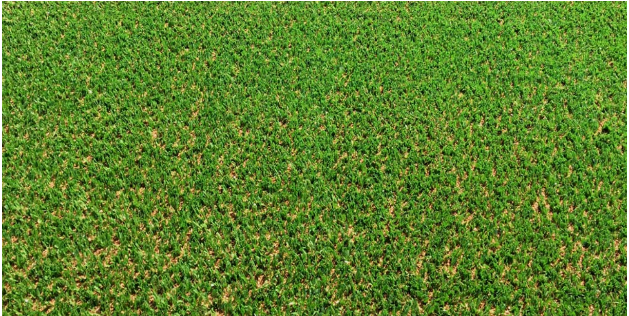
Granular Cork infill material is lighter in color and weight than traditional black SBR Crumb Rubber
