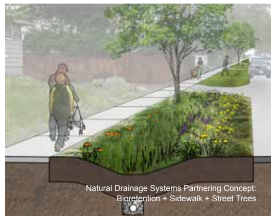
Roadside bioretention installed for Stormwater Code Compliance
