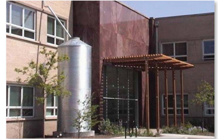
An example of design incorporating stormwater cistern
