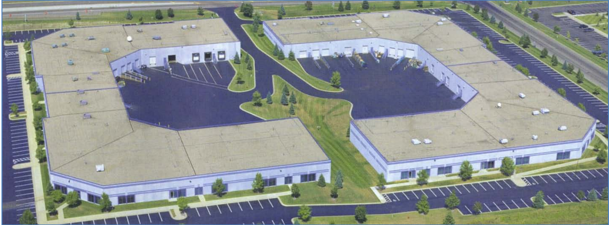
Figure 50: Site design of incubator building type with interior loading area. 212 This particular design shields loading from the surrounding neighborhood, but would have to be altered to provide a better walking environment.
