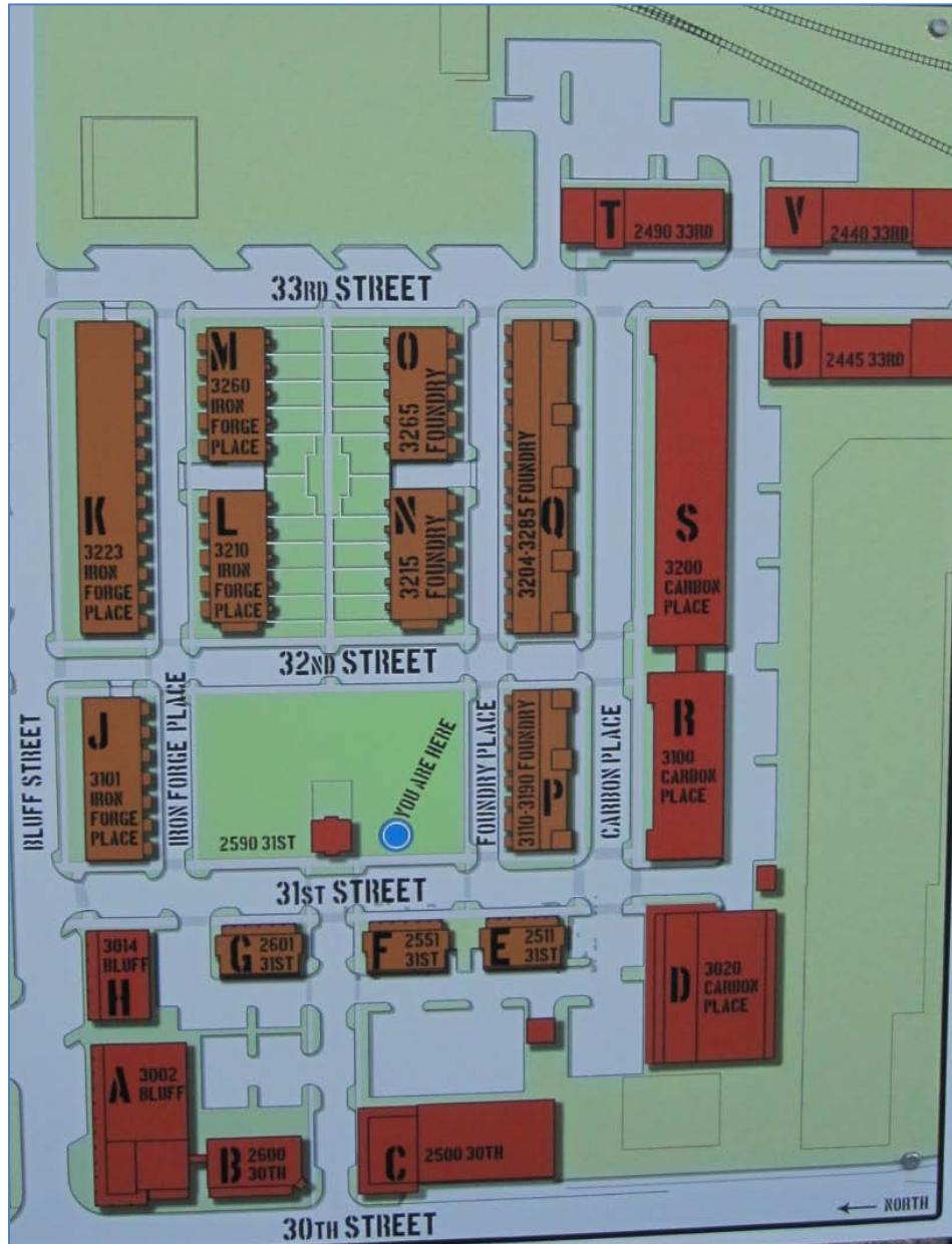
Figure 68: Steel Yards map. Note that residential buildings (E, F, G, J, K, L, M, N, O, P, and Q) are sheltered from arterial by office/retail (A, B, C, and H) and office-only (D). Also note that industrial buildings (R, S, T, U, and V) are closest to train tracks and neighboring industrial uses.
