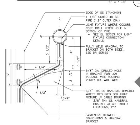
HANDRAIL BRACKET DETAIL
