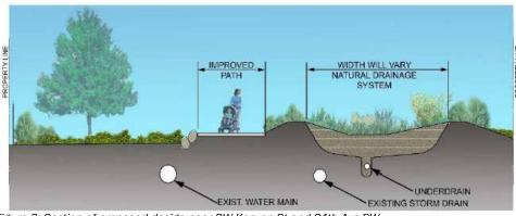
Figure 3: Section of proposed design near SW Kenyon St and 24th Ave SW
