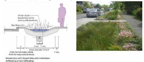
Figure 4: Example of Natural Drainage System with side slopes along street edge.
