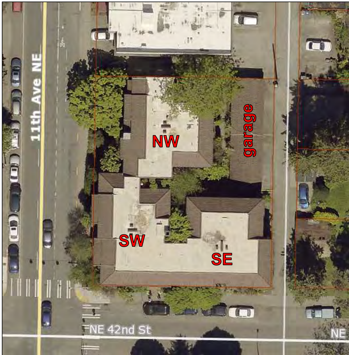
Fig. 3 – Orientation key, showing NW, SW, and SE building masses. North is up. Although connected on the exterior, each of the three building masses are not connected on the interior and function separately. Each is accessed from point entries on the street, accessing a front main stairway, typically serving two units per floor. Each also has a separate rear stairway, accessible from each unit, accessing the rear courtyard. The separate, freestanding garage is noted at the northeast corner. Faint red lines indicate tax parcel boundaries. (KCTA)
