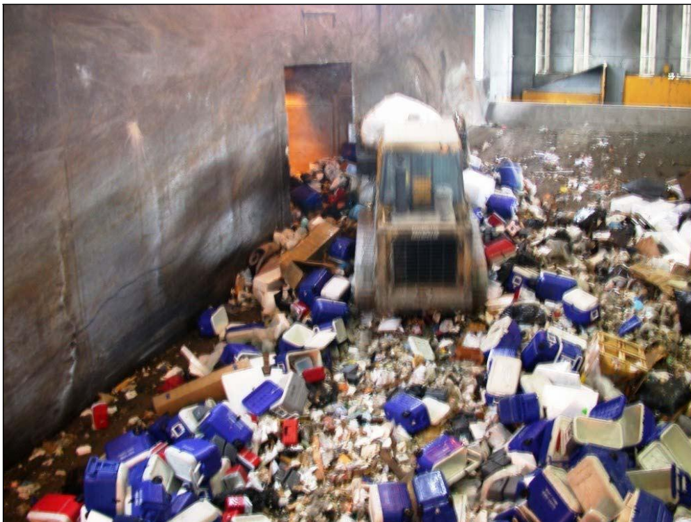
Fig. 26: Bulldozer pushing materials through a hole in the interior east side of the west wall into the hopper above the hydraulic compactor unit. This wall was altered to accommodate the new use of intermodal shipping containers in 1991. (March, 2008)
