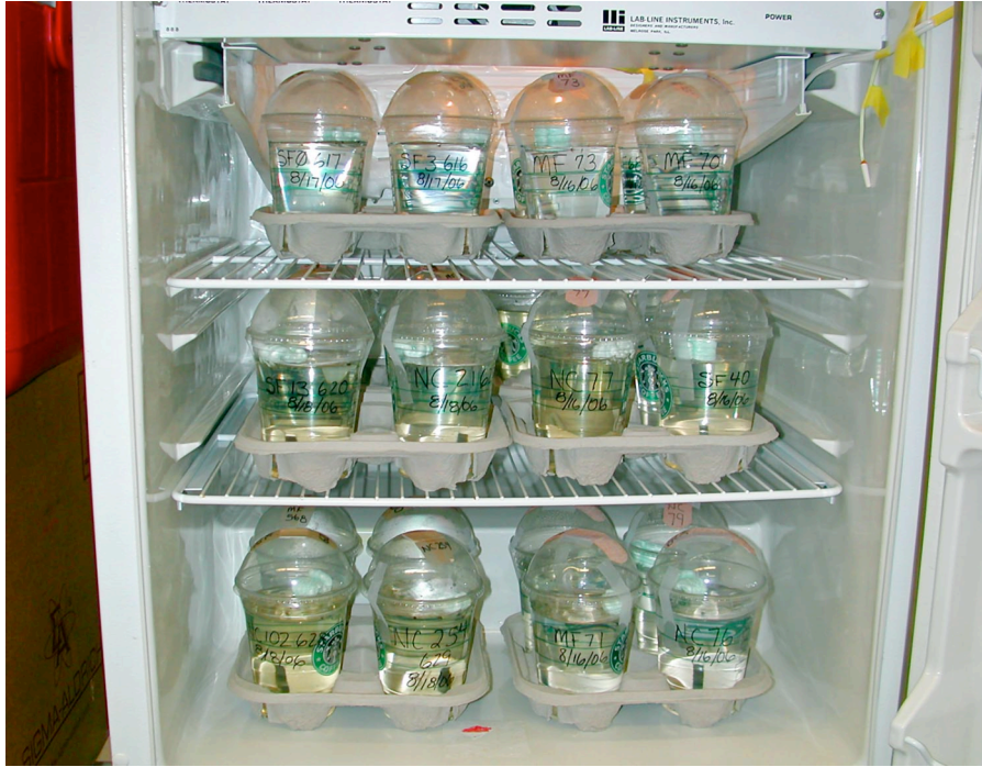
Figure 8. Incubation cups and chamber for assessing the efficacy of methoprene for controlling the production of mosquitoes in catch basins in Seattle. Pupae were incubated for 4 days at 24-26 C to determine percent emergence.
